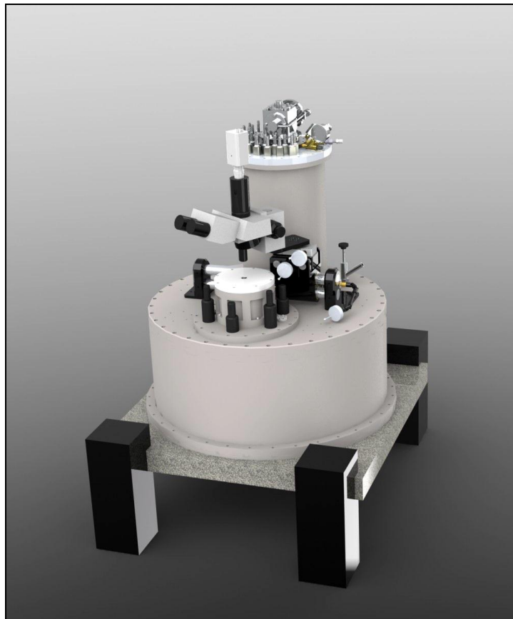
The inverted SQUID microscope, shown with optical microscope and cryocooler
