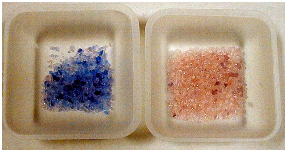
Figure 42 Silica Gel Indicator Colors
