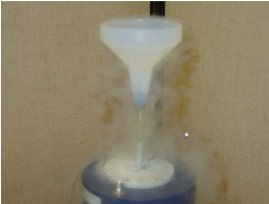
Figure 12 Adding Liquid Nitrogen to a Cold Dewar
