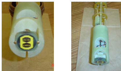
Figure 7 SMM-701G probe in the “horizontal” orientation
