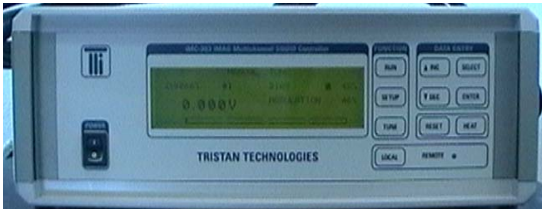
Figure 3.6 Model iMC-303 Cryogenic Control Unit
