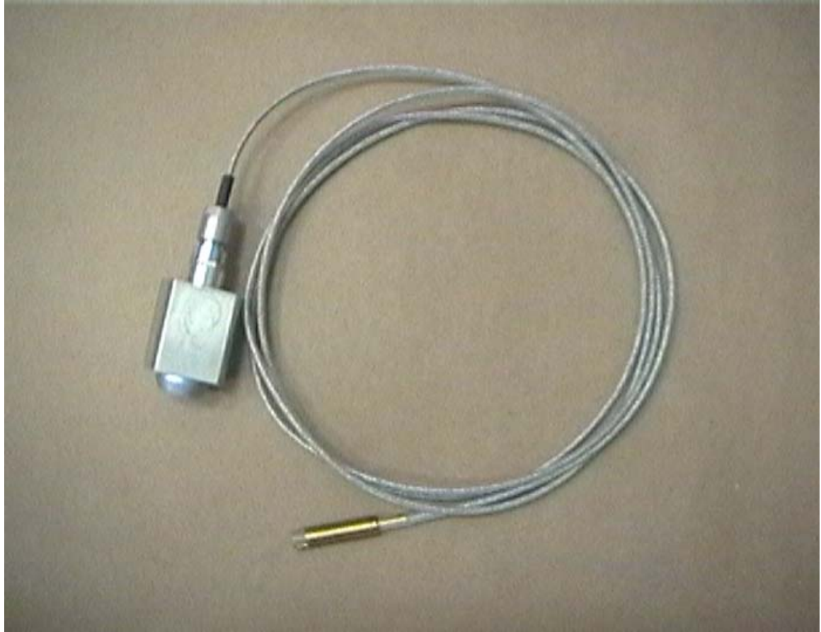
Figure 2.3 Typical Custom Length Cryogenic Cable
