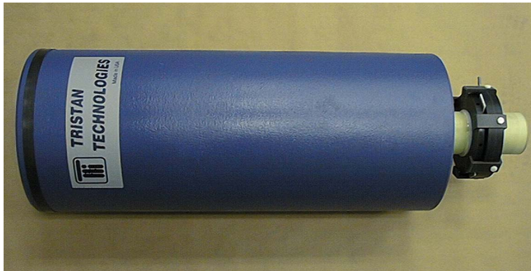
Figure 2.1 Model BMD-9AT Liquid Helium Dewar
