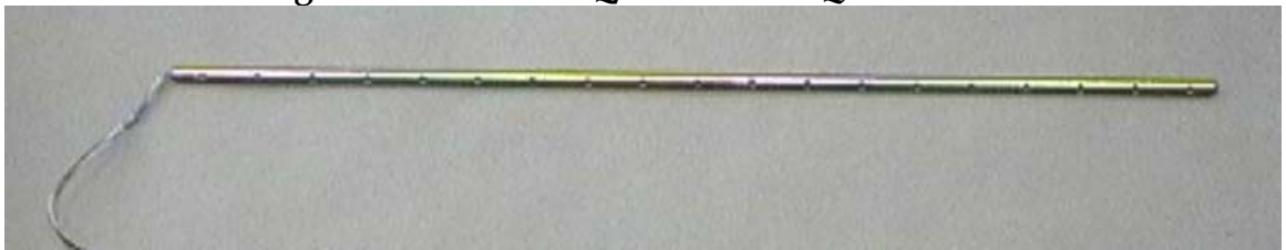
Figure 3.2 Liquid Helium Level Sensor
