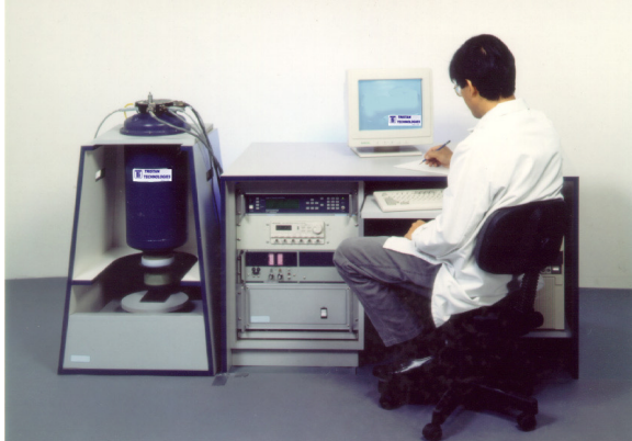
Model SMM-601 Scanning SQUID Microscope with dc and ac biasing magnets
