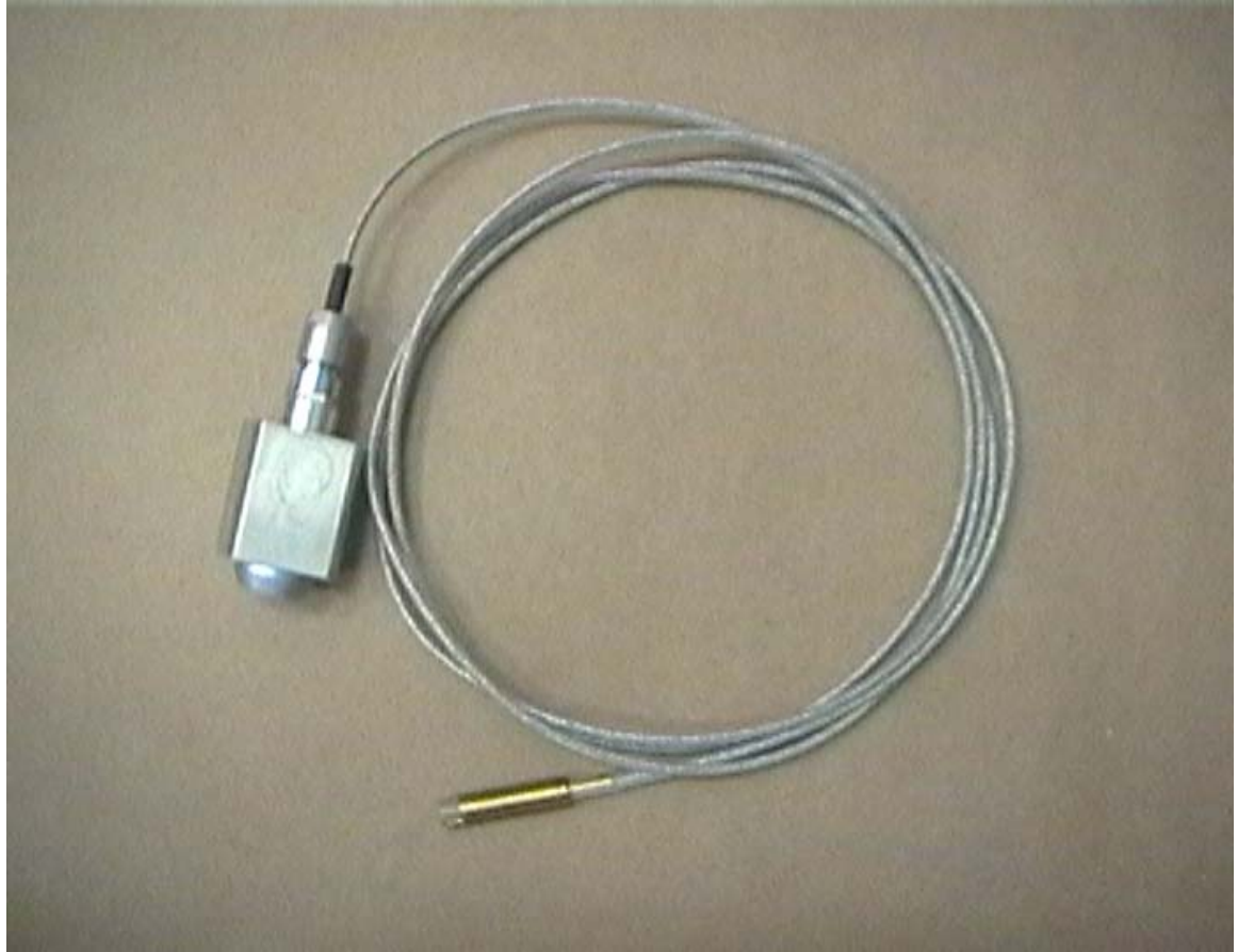
Figure 2.3 Custom Length Cryogenic Cable
