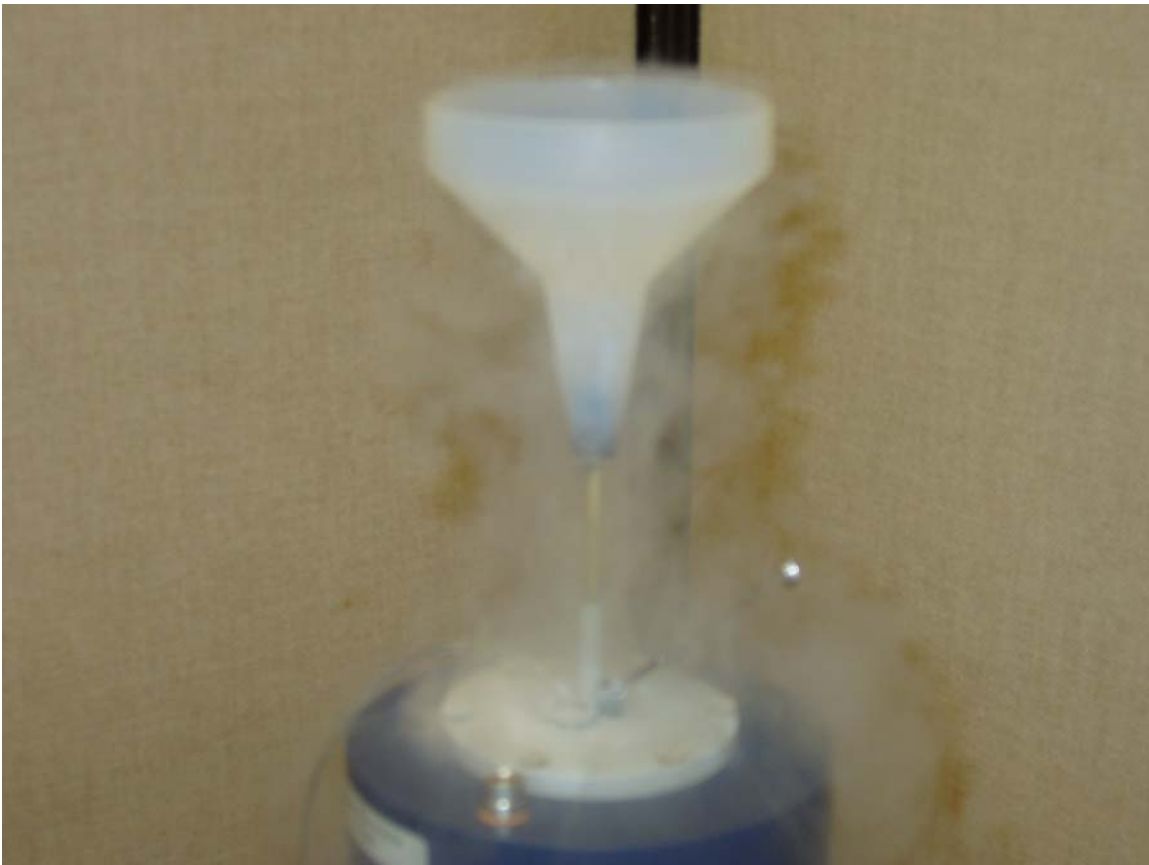
Figure 12 Adding Liquid Nitrogen to a Cold Dewar
