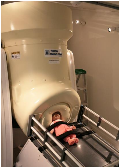
Image of representative baby head in the MAGView helmet
