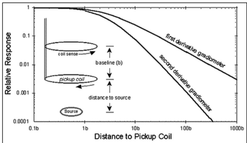
Figure 3: Response of gradient coils relative to magnetometer response (1/r<sup>3</sup> suppressed)
