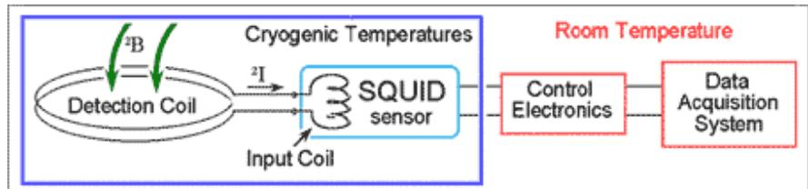
Figure 2: Block diagram of a SQUID magnetometer
