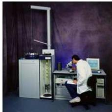
Model SMM-1000 Scanning SQUID Microscope
