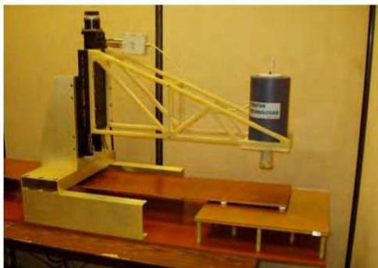
Figure d: SMM-701 NDE scanning system
