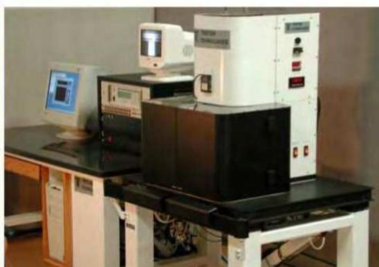
Model SMM-770 Scanning SQUID Microscope
