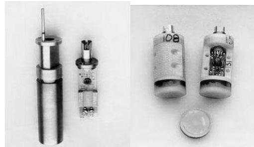
LTS SQUID sensor HTS SQUID sensor
