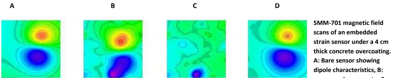
SMM-701 magnetic field scans of an embedded strain sensor under a 4 cm thick concrete overcoating. A: Bare sensor showing dipole characteristics, B: sensor under concrete, C: bare concrete. Image D = B – C is a digital subtraction of B and C showing that it is possible to image objects deep underneath magnetically complex coverings. The scans cover a 6 cm x 6 cm area.
