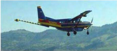
Figure a: Tristan HTS SQUID gradiometer in flight
