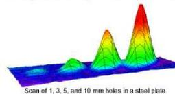
Scan of 1, 3, 5, and 10 mm holes in a steel plate
