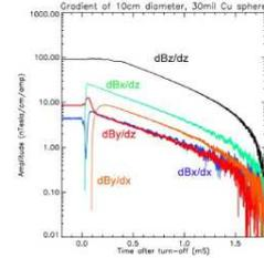
Data from Controlled Source Measurement of a 10 cm diameter hollow (30 mil thick) copper sphere showing data from the five independent tensor gradients. Data was collected at 1 msec intervals.
