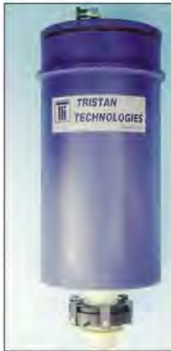
Fig. 1. Dewar with adjustable dewar tail mechanism shown at bottom
