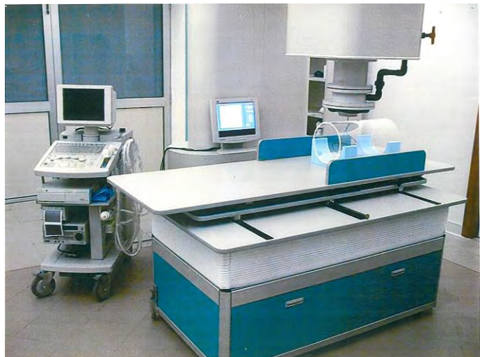
(Left) Installed model 663 spine system dewar , showing pneumatically assisted x-y, and z- orientation control. (Center) Dewar insert, with array of 71 channels plus reference channels. (Right) Control electronics rack for 108 kSample/sec data acquisition and RAID arrays for simultaneous monitoring, storage, and data upload.
