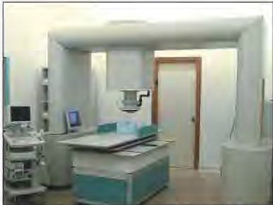
Fig. 3. Ferritometer ® system with patient bed and computer control system shown. The system operates without a magnetically shielded room.
