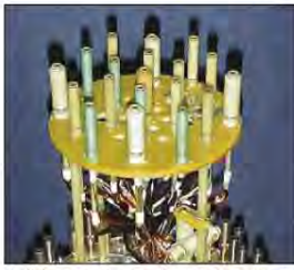
Fig. 3. 19 sensor position system for intestinal measurements, showing partially populated array. This insert is upgradeable to 37 sensor positions.
