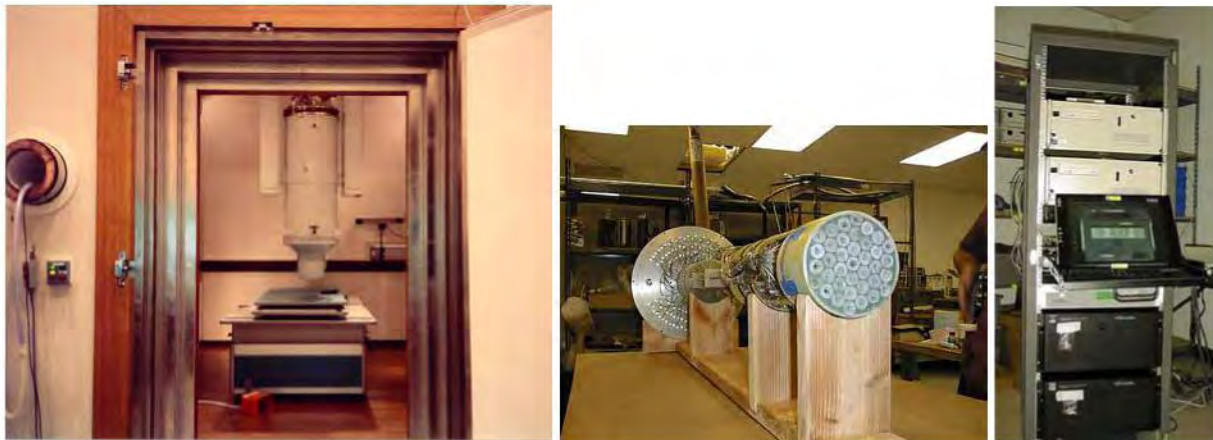
(Left) Installed model 663 spine system dewar , showing pneumatically assisted x-y, and z- orientation control. (Center) Dewar insert, with array of 71 channels plus reference channels. (Right) Control electronics rack for 108 kSample/sec data acquisition and RAID arrays for simultaneous monitoring, storage, and data upload.
