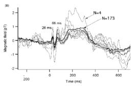
Somatic evoked magnetic field (SEF) obtained from a 7-month old as a function of number of averages from N=4 to 173 epochs. The waveforms are the differences of the SEF at two field extrema. This shows that a small number of averages are needed to acquire SEF data. (data acquired using a Tristan babySQUID<sup>®</sup> system).
