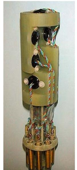
T877 sensor housing showing cold electronics
