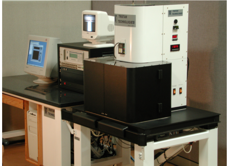
Model SMM-770 Scanning SQUID Microscope with dc and ac biasing magnets
