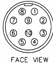
Figure 18 iFL-301 Pigtail Connector Pinout ( Face View )
