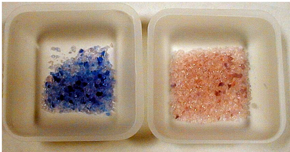
Figure 12 Silica Gel Indicator Colors
