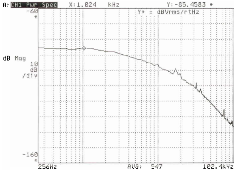
Figure 6 SG40324 noise measured at Tristan
